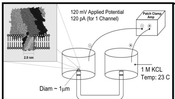
**Figure 1. Schematic diagram of the nanopore transduction detector.** The nanopore detector consists of a single pore in a lipid bilayer that is created by the oligomerization of the staphylococcal alpha-hemolysin toxin, and a patch clamp amplifier capable of measuring pico Ampere channel currents.
