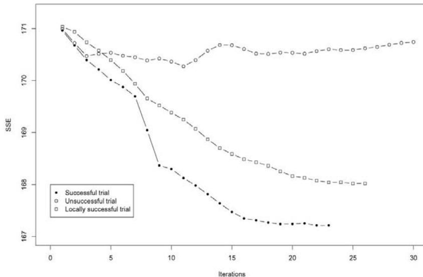
**Fig. 15a.** Training history on SSE for three types of clustering result: successful, unsuccessful; and locally successful.
